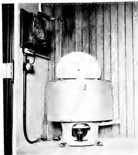
FIG. 52.—Electric centrifuge made by the International Instrument Company, Cambridge, Mass.
